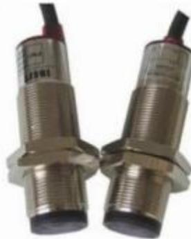
D、 Cylindrical reflective photoelectric switch: (role with the above) a total of three lines, of which two lines power transmission In, brown: + 12V, blue: GND and 1 line signal output (black), when people pass reflected Type photoelectric switch (reflection distance of 10-20mm) output +12 V, otherwise 0V
