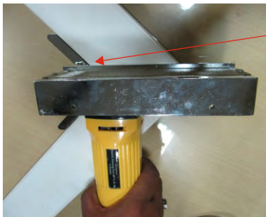
V Corner Cleaning Tool Model SP TL EL 05
